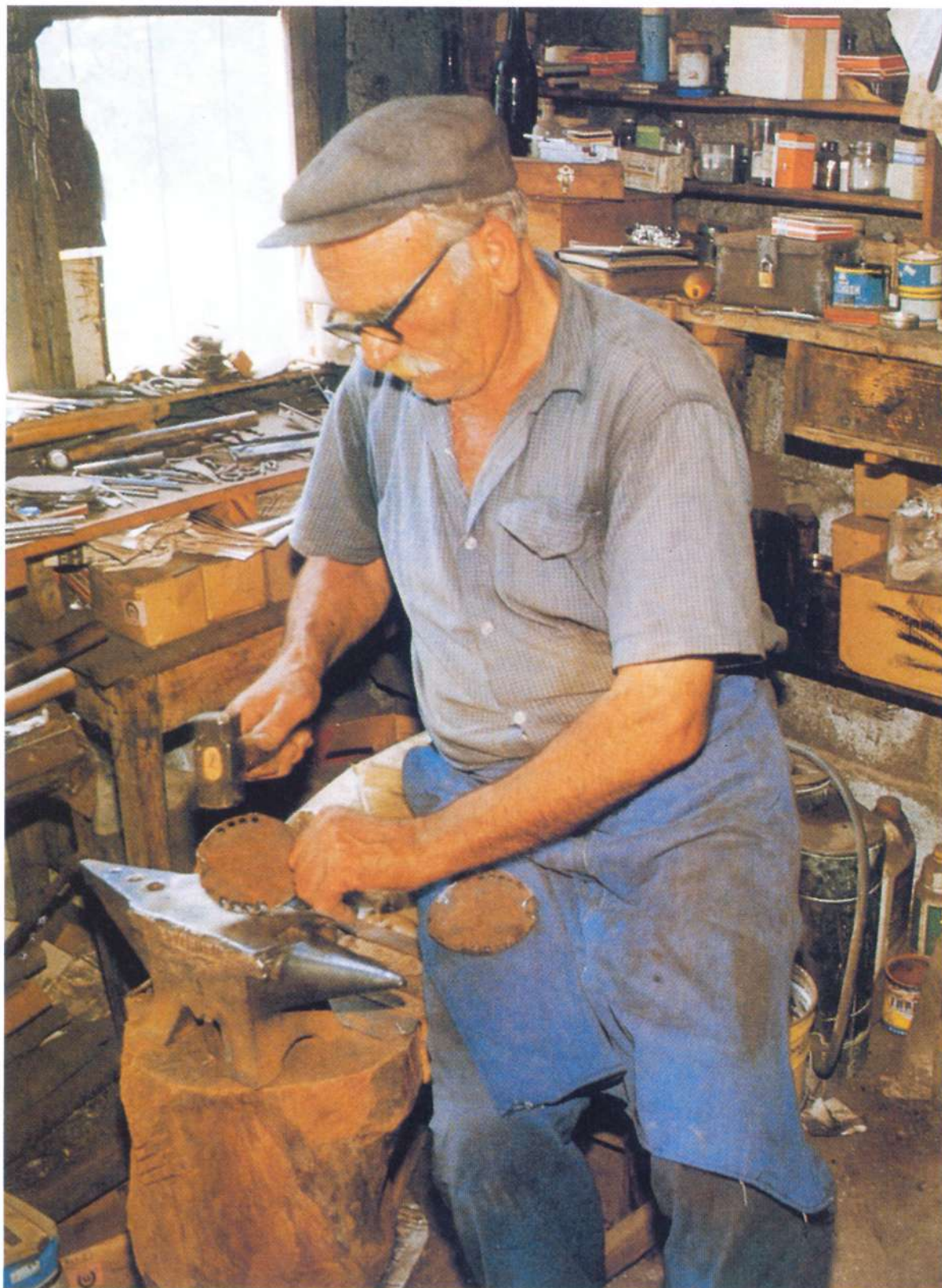
The local farrier, Yiannis Ghekas making a flat plate in his workshop (Photograph taken 1986)
