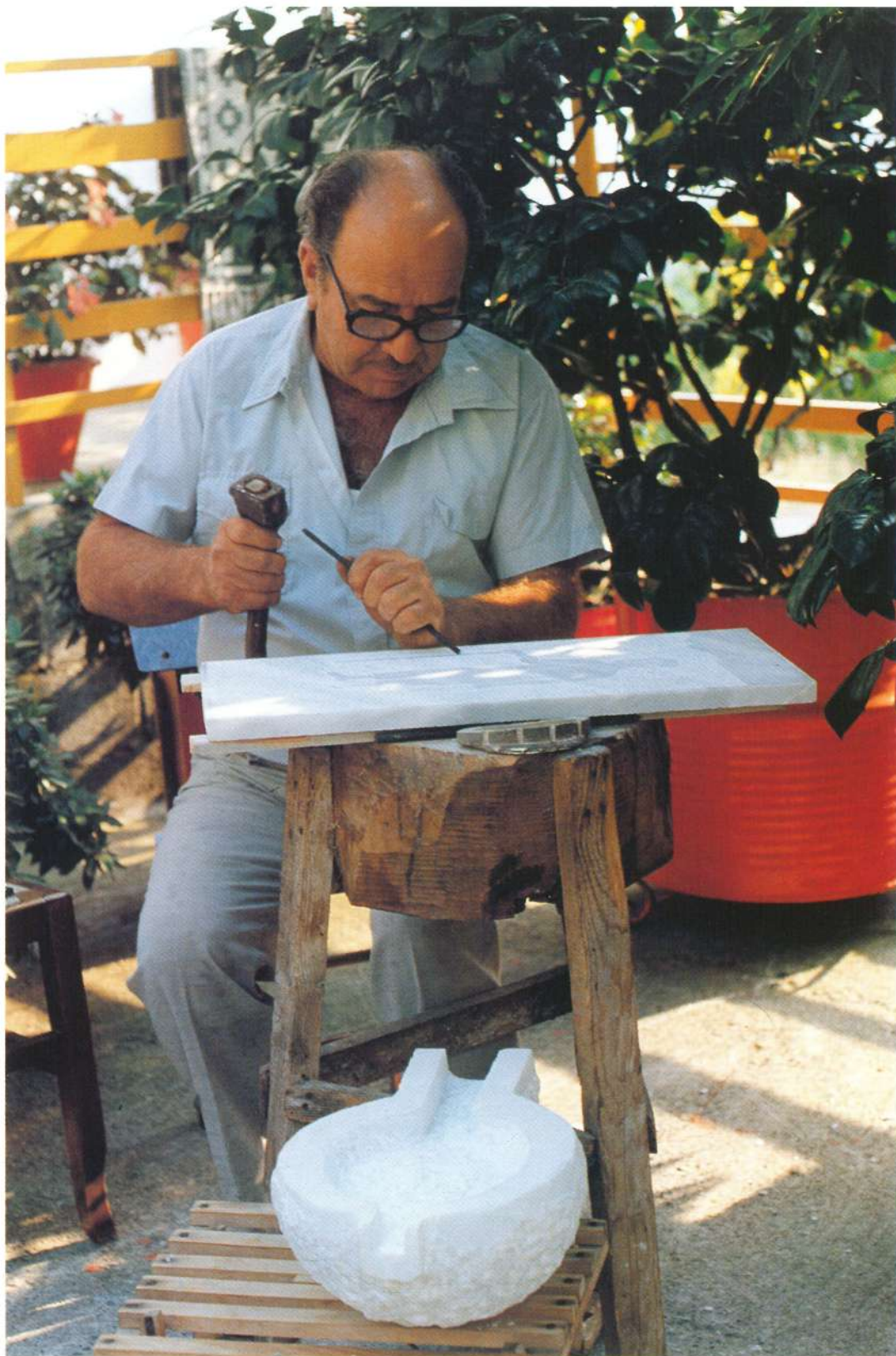
Panayiotis Demou carves traditional designs on a marble slab with a chisel and hammer; nearby a completed fountain basin (Photograph taken 1986)
