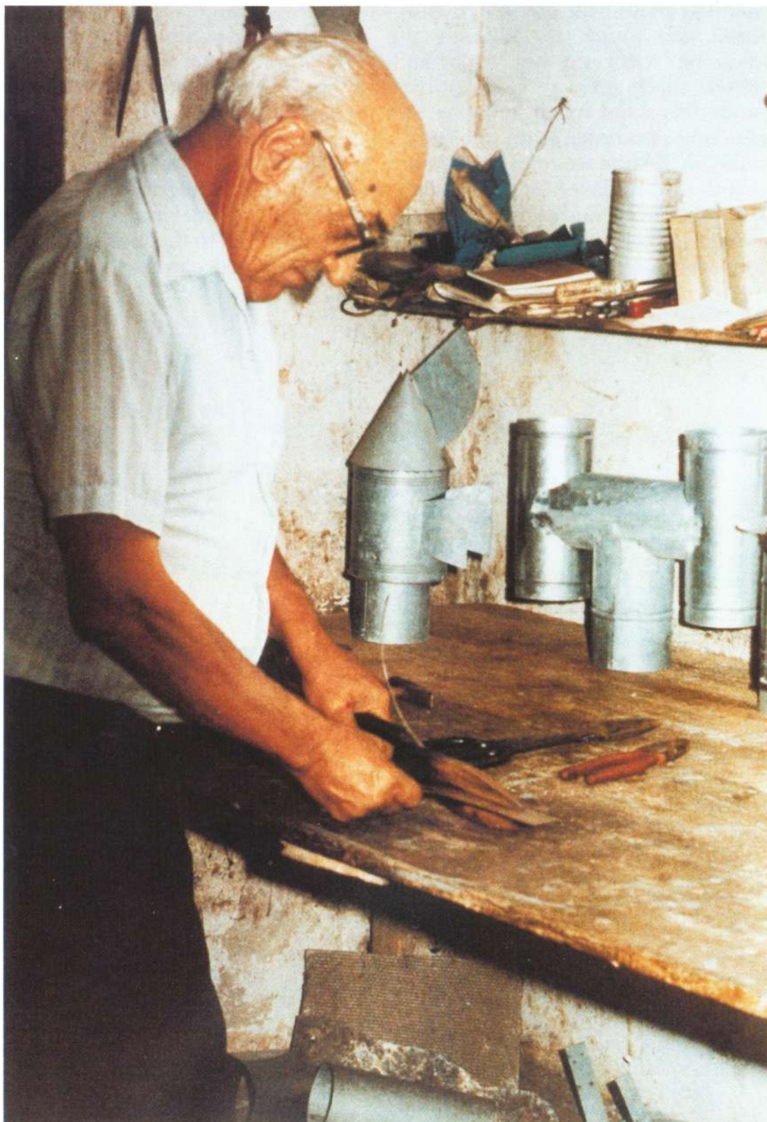
With tinsmith's scissors, Nikos Tsangarakis cuts a tin plate in his workshop (Photograph taken 1986)
