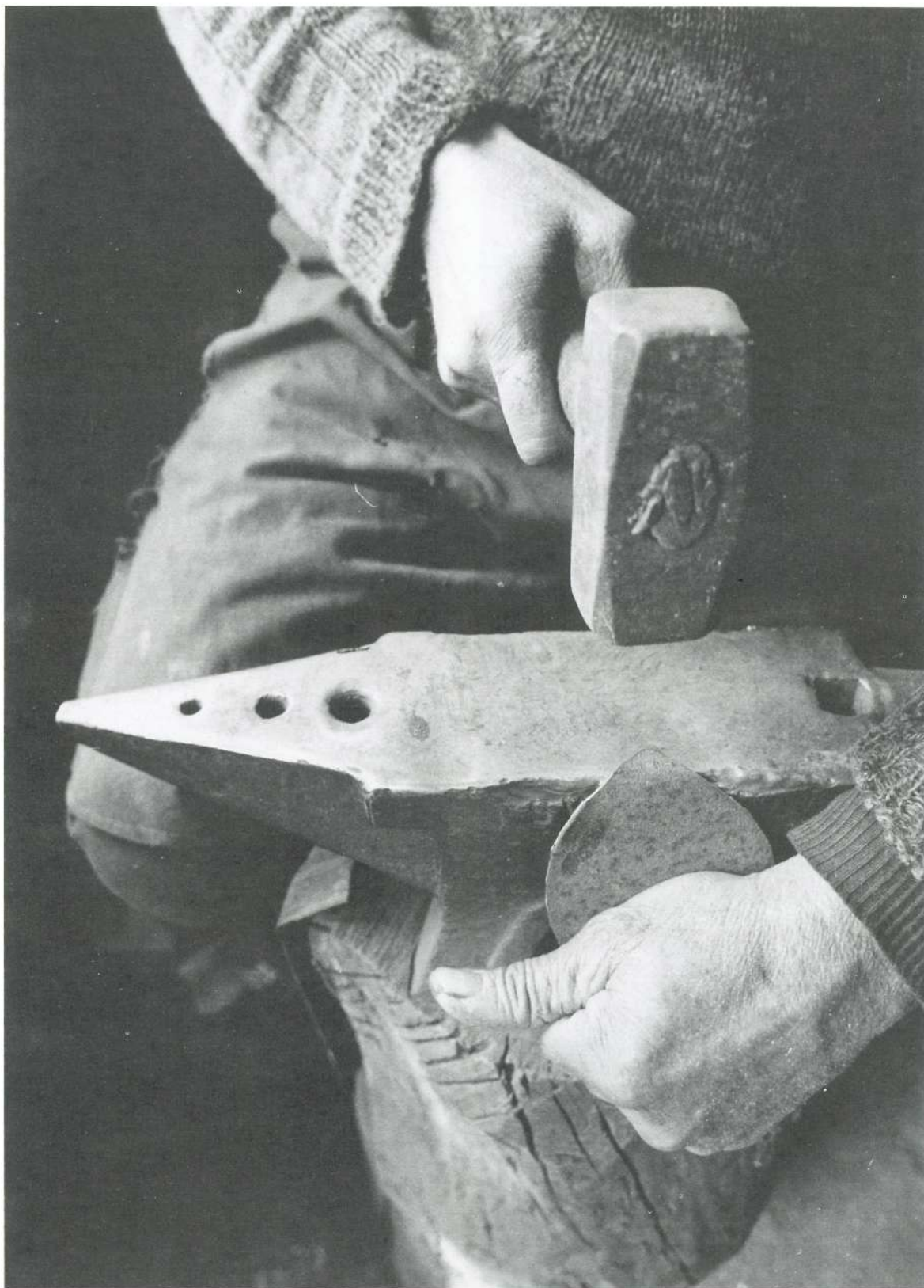
Every flat plate must have a clip on the front to grasp the hoof firmly (Photograph taken 1986)
