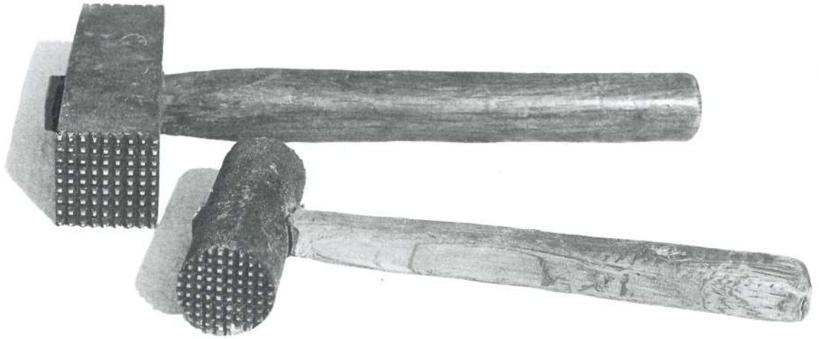
Stone carver's tools, for etching designs on stone (Photograph taken 1986)
