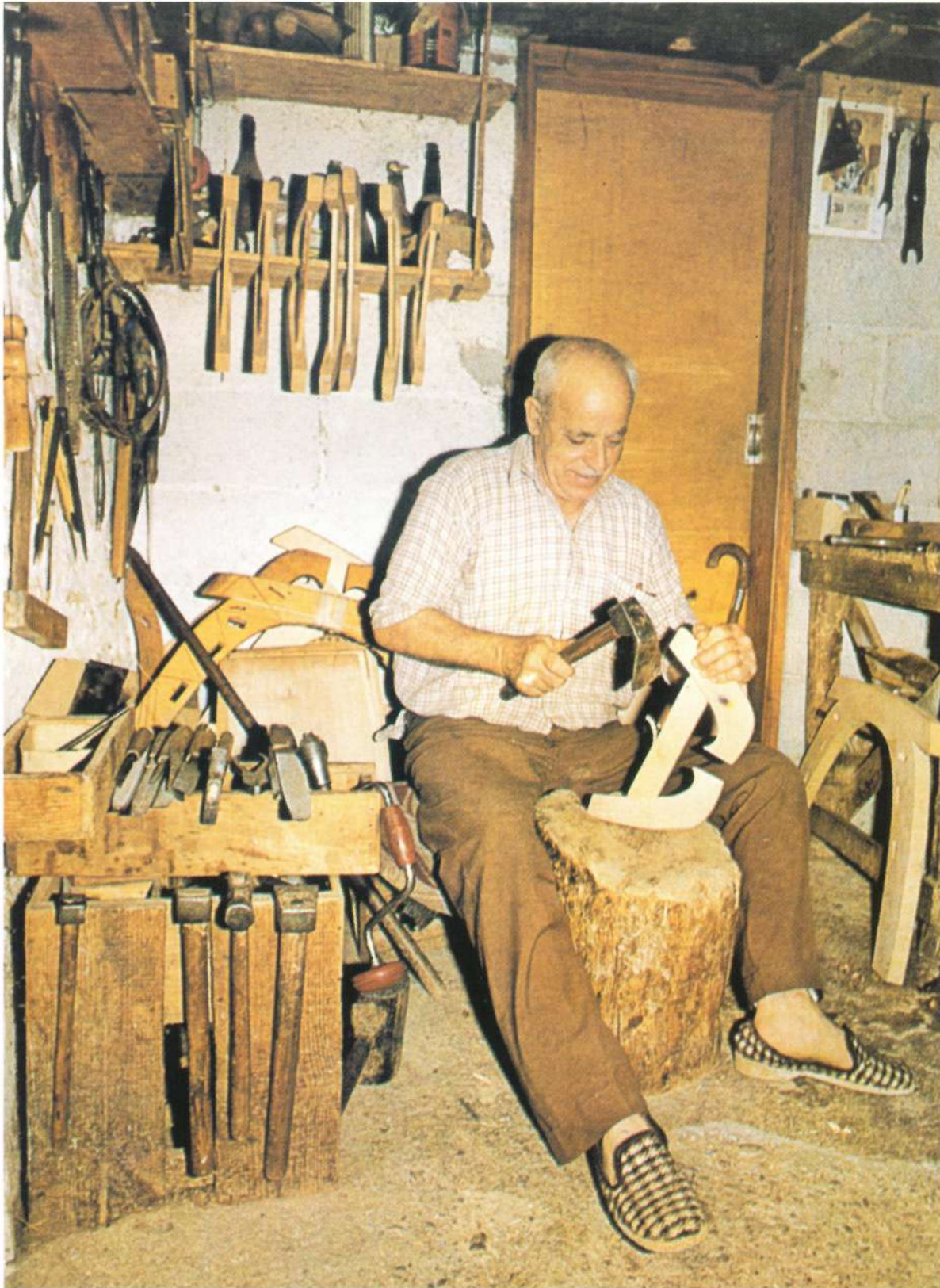
Vangelis Katardzis, local packsaddler in his workshop, carving a wooden frame for a packsaddle (Photograph taken 1981)
